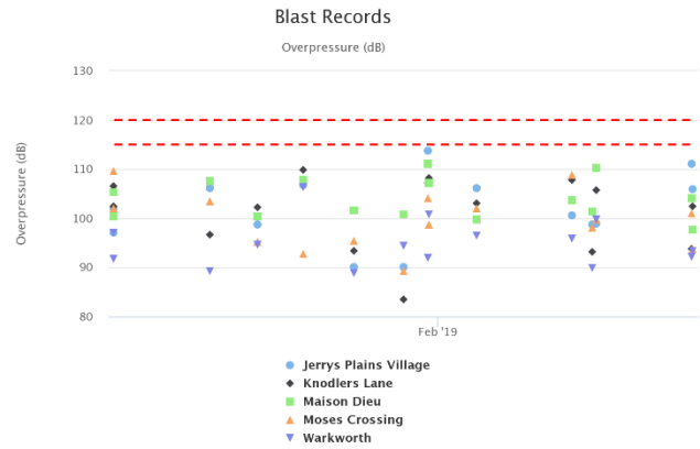
Figure 10: Overpressure Blast Monitoring Results – February 2019
